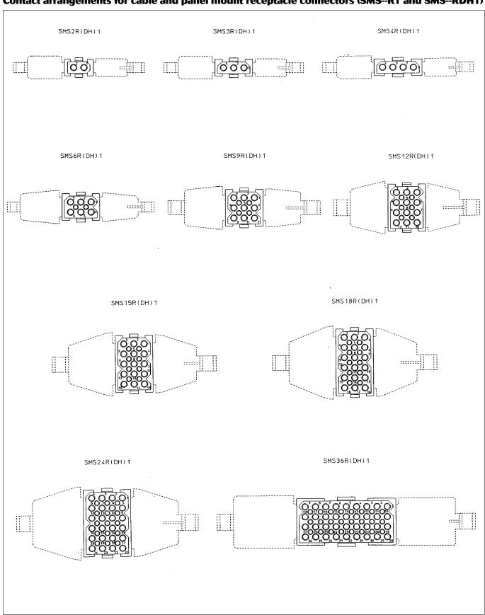
Contact identifications shown are for mating face. Contact identifications of wiring face are identical as shown on the plug arrangements
