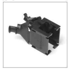
Separate strain relief hoods are available for all standard plugs SMS—P1. The hoods consist of identical halves that snap into position on the plug and are secured in place with the cable tie drawn tightly around the cabe entry collar.
